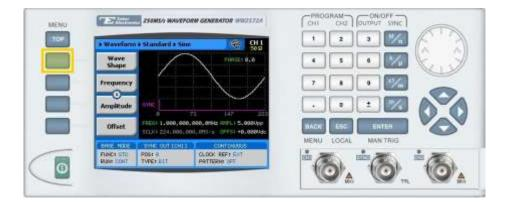
2. Select one of the wave shapes from the list box using the dial or the cursor keys, and press ENTER.
